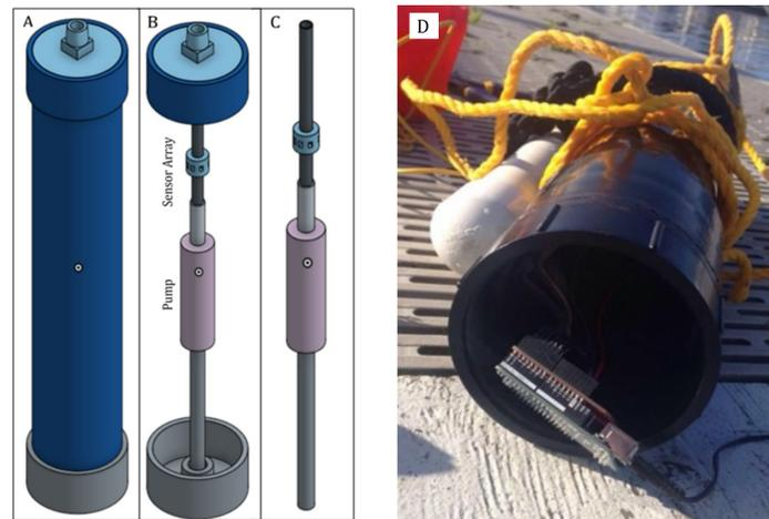
Figure 1 Digital rendering of m-PARR (A-C) showing the simplicity of the instruments design and (D) the current prototype.
