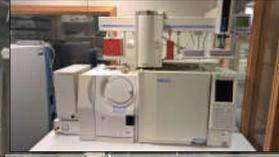
Fig. 4 - Shimadzu Optima 2010 GCMS coupled with Lab Frontiers EGA/PY 3030 two step pyrolyzer and 48 well autosampler
