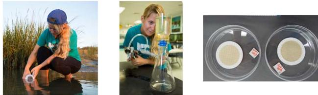
Citizen scientists collect 1-liter water samples and filter them through 0.45 µm gridded filters. They then observe the filters at 40X magnification using a dissecting microscope. Fibers are tested by heating them over a candle flame and observing to see if they are singed (natural) or if they melt into a blob (plastic). Fragment identification is primarily made through feel of the object in the forceps.
